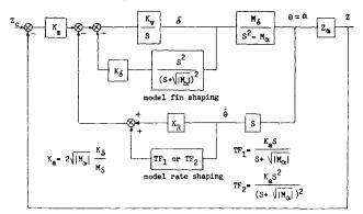
Fig. 1 Lateral acceleration control autopilot using the angular acceleration model.
